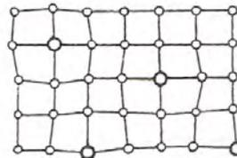
Lattice distortion in a substitutional system.
